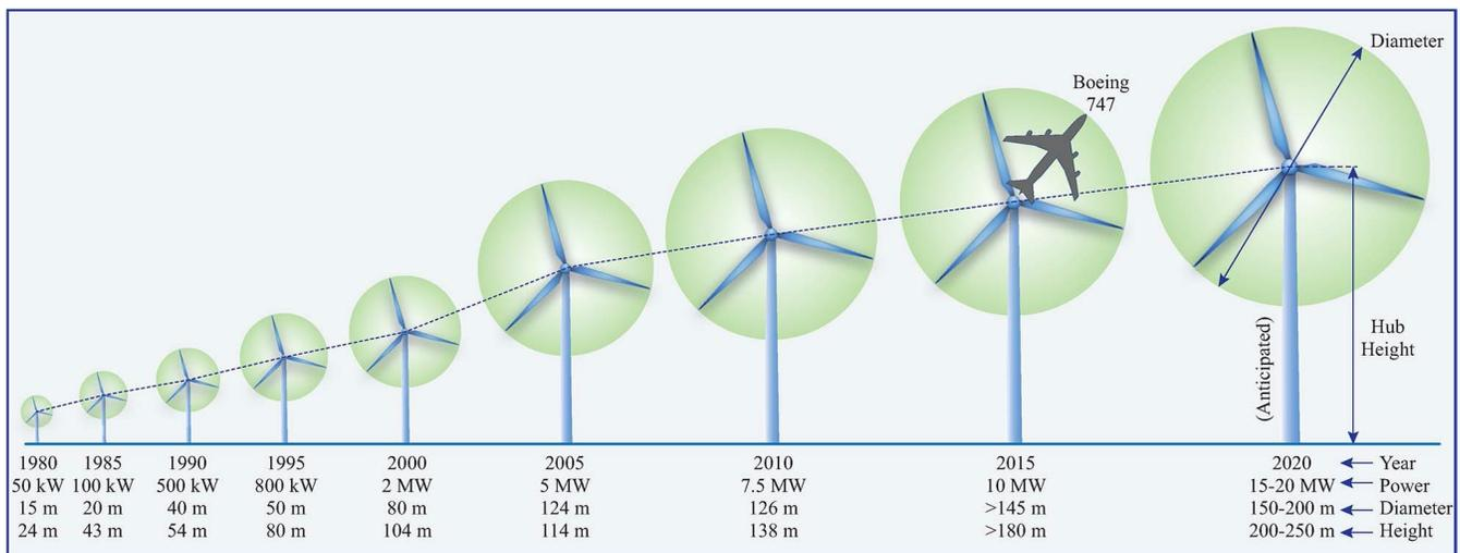
Fig. 1. Evolution in the size of commercial wind turbines.
